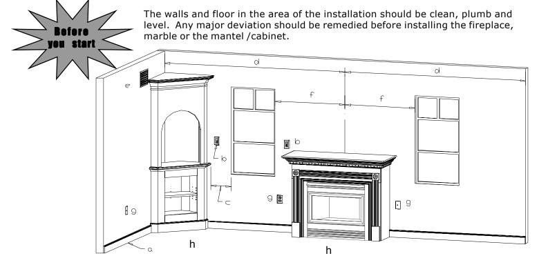
Above is a diagram of issues that may prevent an installation of wood products around a firebox:
